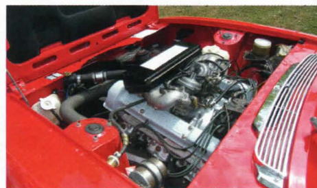
Freshly rebuilt engine has new viscous and Kenlowe fans
